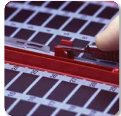
Step 3: Slide backward until blade drops safely into box.
