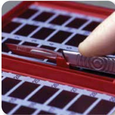
Step 2: Slide forward until blade “catches.”
